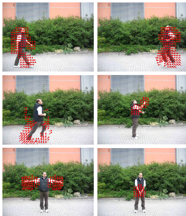
Figure 2: Flow estimation results for a video sequence showing a single person performing various actions, i.e. walking, jogging, boxing, waving, and clapping from left to right and top to bottom, respectively.
