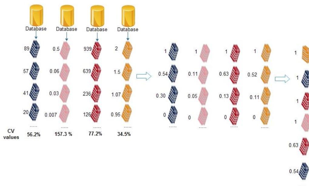
Figure 1.2. The diversified MinMax score normalization. Given a user’s query to four different information sources, each produce ranked lists of documents whose relevance scores are not comparable across lists. MinMax normalizes the scores in each list to the range (0..1). Then the documents from all lists are combined and ranked by their normalized scores (with similar score values pruned by CV)
