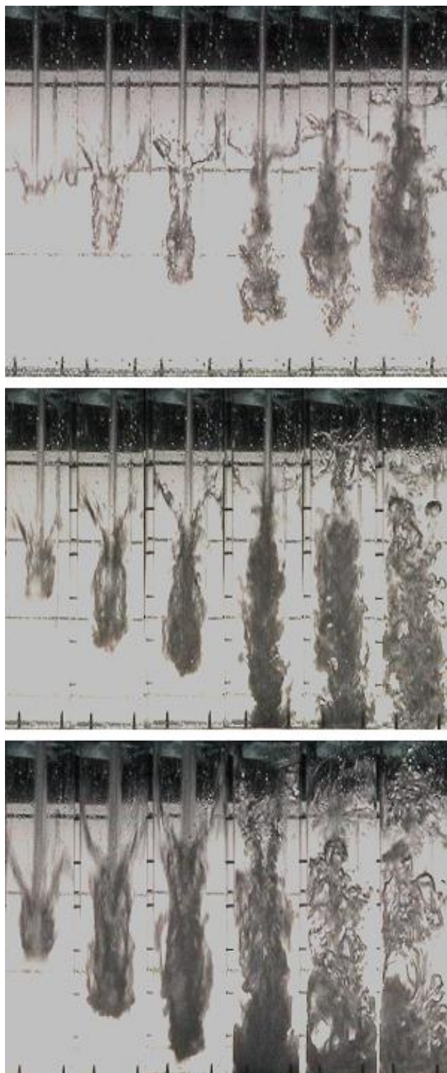
Fig.2. Features of a jet penetration into the pool: experimental data for initial velocity 4m/s, 6m/s, 9m/s, respectively (from the top to the bottom)
