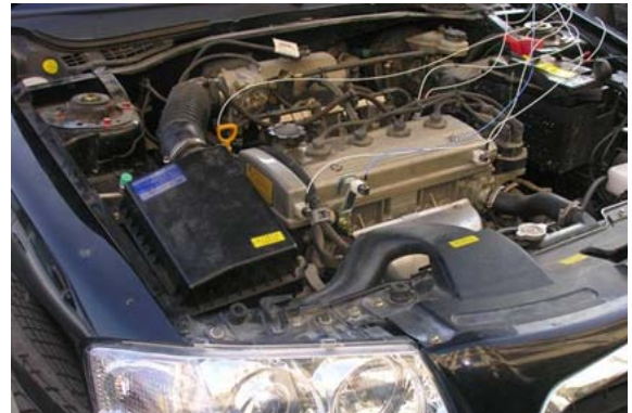
Fig. 10 Test environment and real operating status of powertrain mounting system
