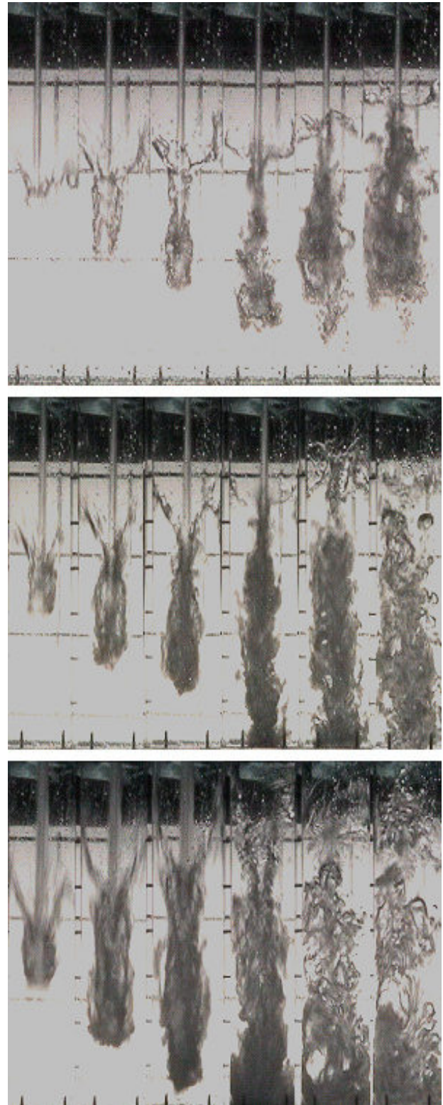
Fig.1. Jet penetration experimental data: initial velocity of a jet - 4m/s, 6m/s, 9m/s, respectively
