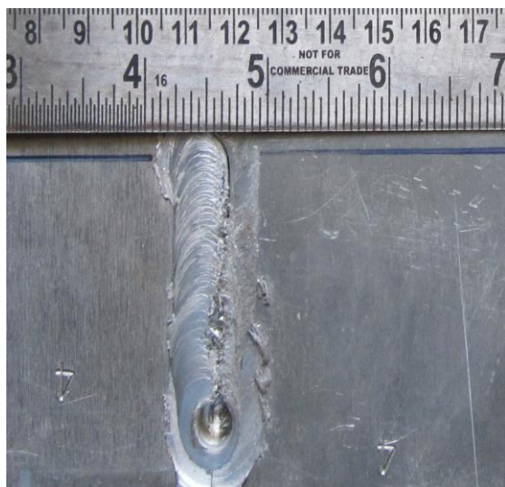
Fig. 2f Incomplete fusion of material
