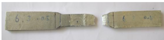
Fig. 2a Failure occurred at 6063 side.
