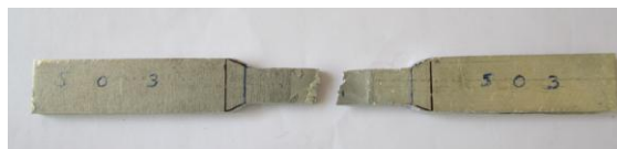
Fig. 2b Failure occurred at the welded region
