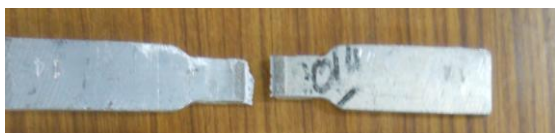
Fig. 2e Failure occurred due to incomplete fusion
