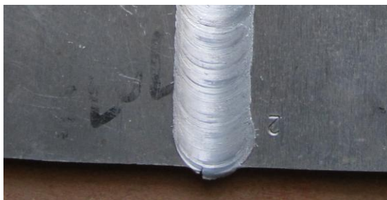
Fig. 2d No skimming of materials at higher tilt angle
