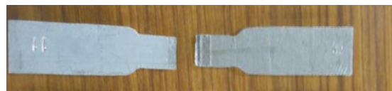
Fig. 2g Failure occurred due to tunneling defect
