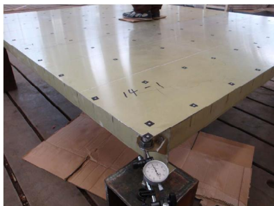
Fig. 12 The experiment of concentrated load applied on the panel.
