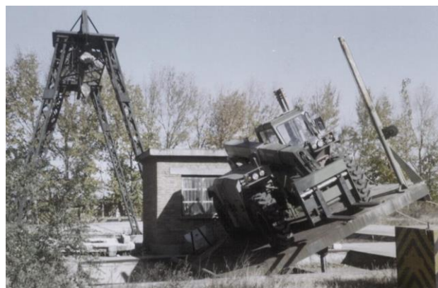
Fig. 11 Platform experiment for lateral stability of telehandlers
