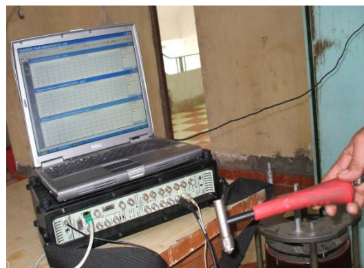
Fig. 4: Main components of hammering test
