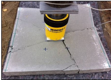
Fig. 5 Failure of the slab
