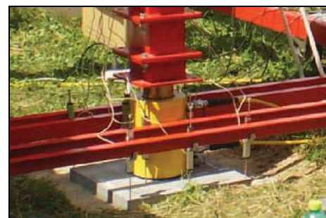
Fig. 4 Load testing of the slab
