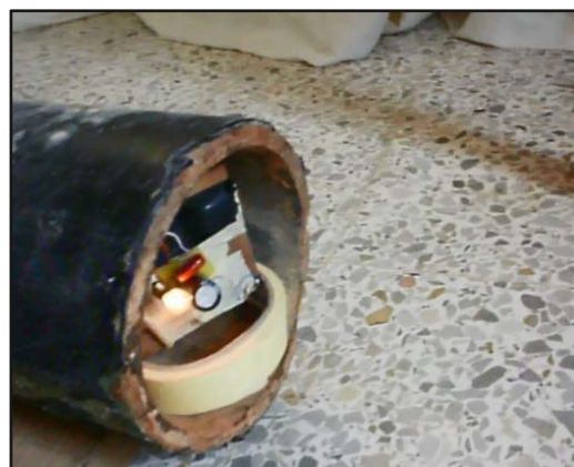
Fig.13. Photo of the rectifier circuit testing inside pipeline with light bulb 12W
