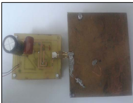
Fig.11. Photo of the PCB harvesting circuit
