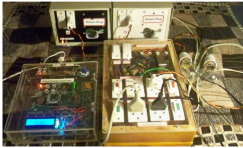
Fig. 17 Test set up showing HEC, Smart Plugs and Smart Grid distribution board
