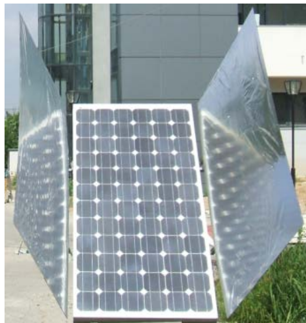
Fig. 16. Prototype of LCPV system realized: a) sketching, b) real system
