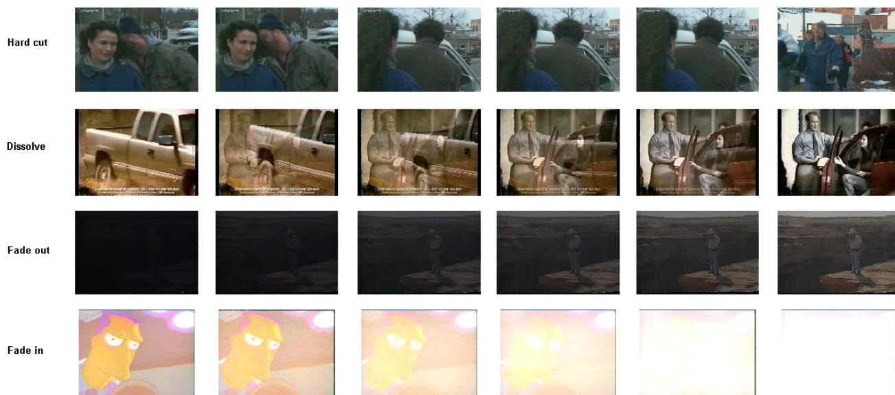
Figure 1: Different type of transitions in a video. First row : hard cut, others : gradual transition
