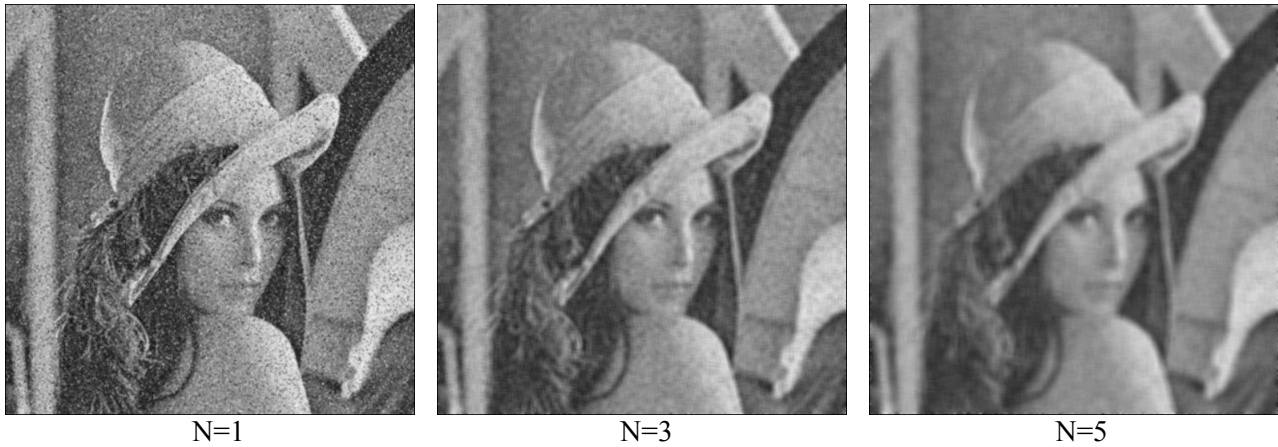
Fig.4 – “Lena” image corrupted by Gaussian ( \sigma=20 ) and impulse noise (prob=10%): results given by (2N+1) \times (2N+1) mean filters.
