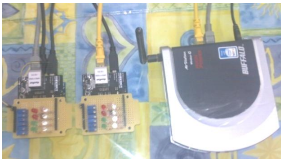
Fig. 10, Two RTU's with Air Station Wireless High Power Module.
