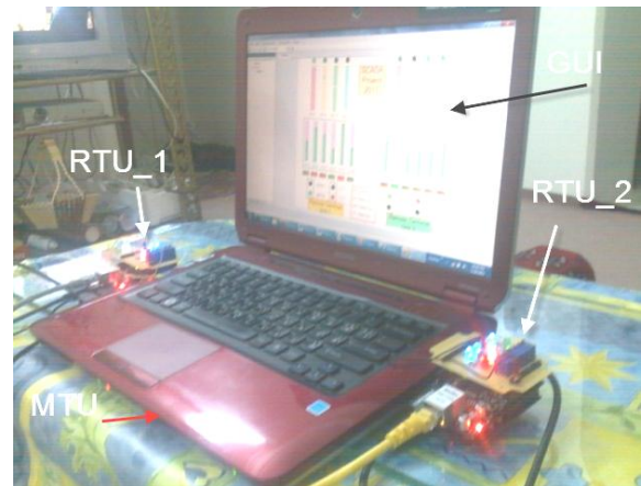
Fig. 11, Two RTU's with MTU in operation mode.
