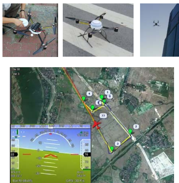
Fig. 17. Set-up and test the trajectory-tracking controller for the autonomous mini quadrotor UAV.
