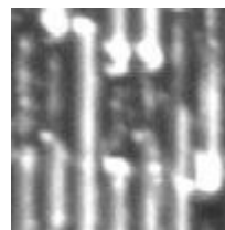
(b) The texture image of a workpiece surface machined with a dull cutting tool
