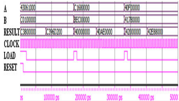
Fig.17: Output waveform of complete 32-bit floating point multiplier
