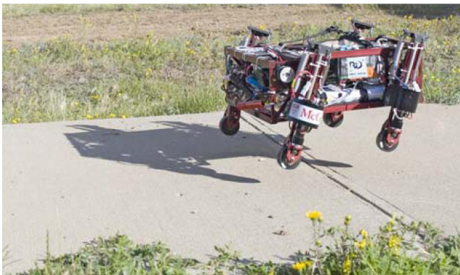
Fig. 3: The PAW robot with bounding gait (Used with permission from [14])
